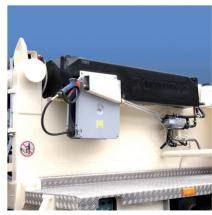
The 600 litre water tank is mounted close to the hopper and can be optionally equipped with a high pressure cleaner or a water tank heating
