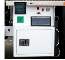
The Command centre on the ground integrates the rear panel control, chamber valve control block, the mailbox for the dockets, and a lockable equipment box.
