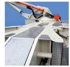
The SX outriggers leave enough space to mount a pump kit with a 2,5m stro-ke. The result is less wear and smooth pumping.
